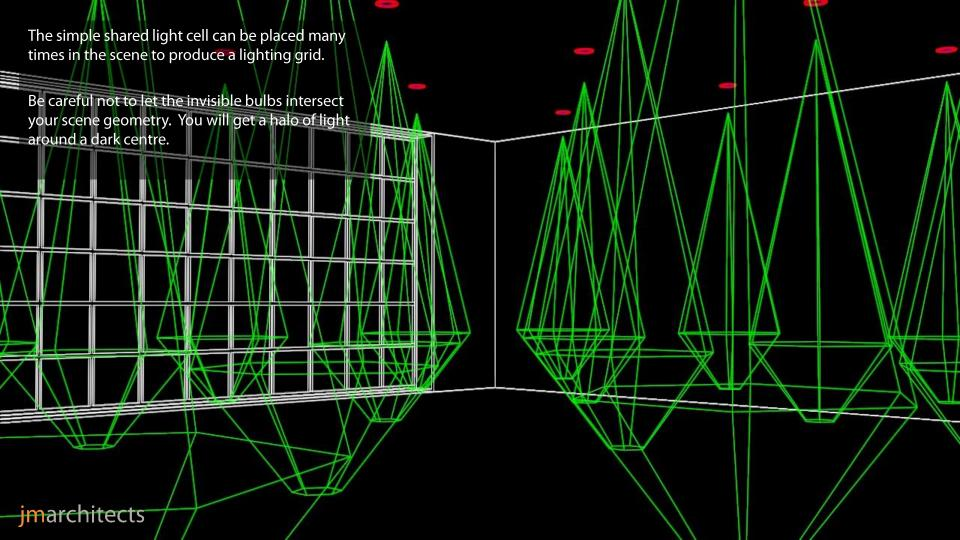
As expected, the result is a brightly lit scene, with lots of ambient light. At this point just a few conventional direct lights can be added to the scene, where the required, to produce sharp shadows, ies profiles, etc. Where light sources have enough surface area the "invisible glow" geometry may not be required.
